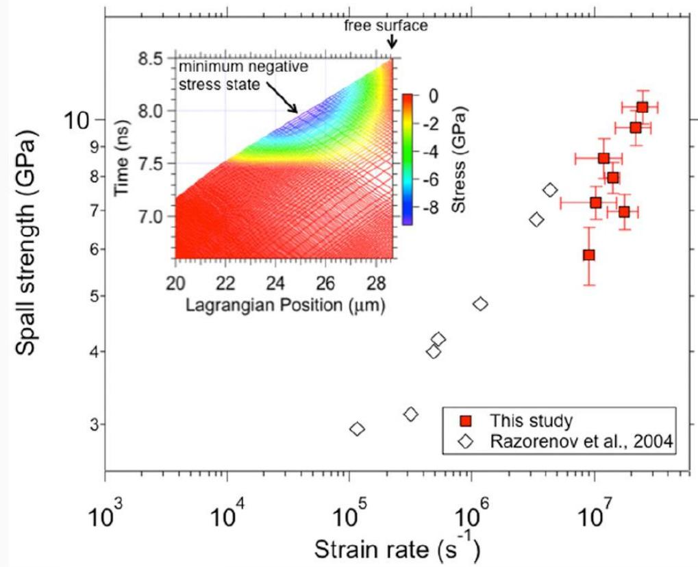
**Spall strength increases with increasing strain rate**
