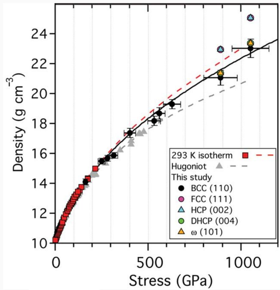
**BCC structure stable to 1050 GPa under ramp compression or until shock melting at 390 GPa.**
