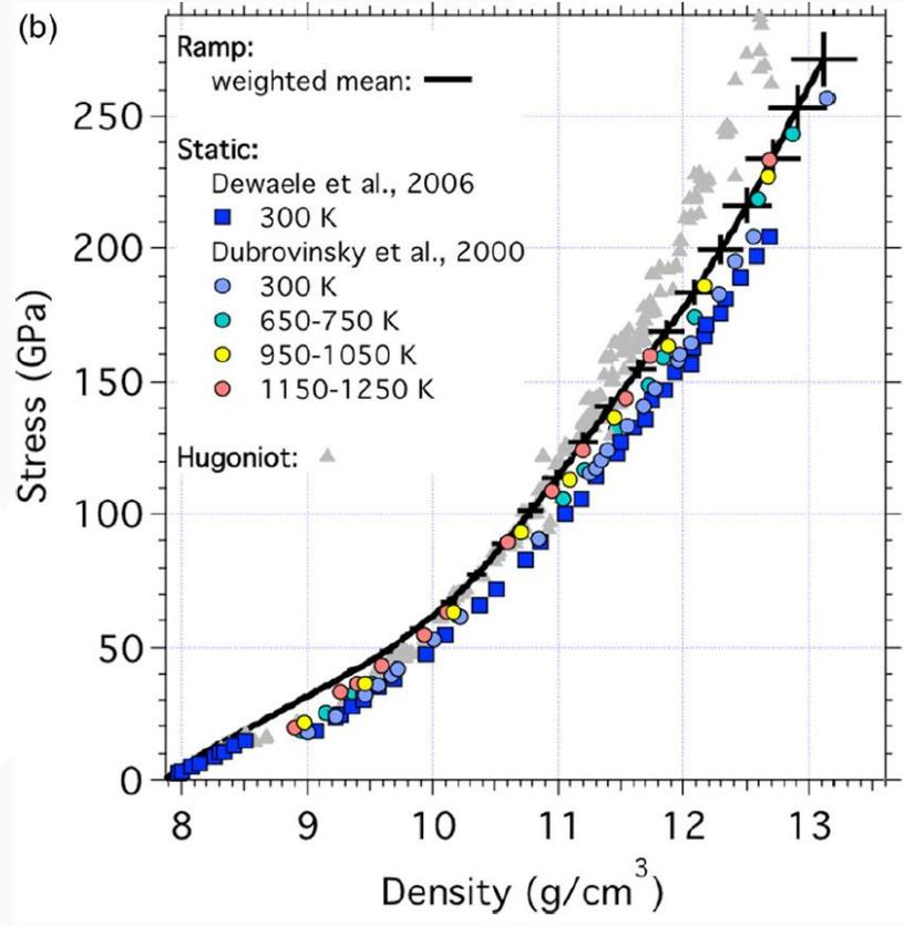
**Data is consistent between shock compression and static DAC data**
