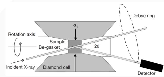
**Strong (hkl) dependence of lattice strain reflects a strong elastic anisotropy**
