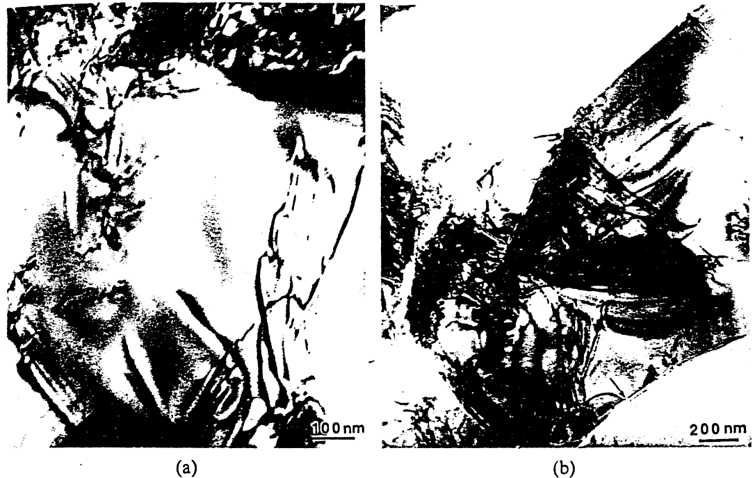
Figure 2.33. (a) Dislocations in alumina after passage of stress waves, (b) cracks in alumina (marked by arrows). [From Louro and Meyers (1989).]
