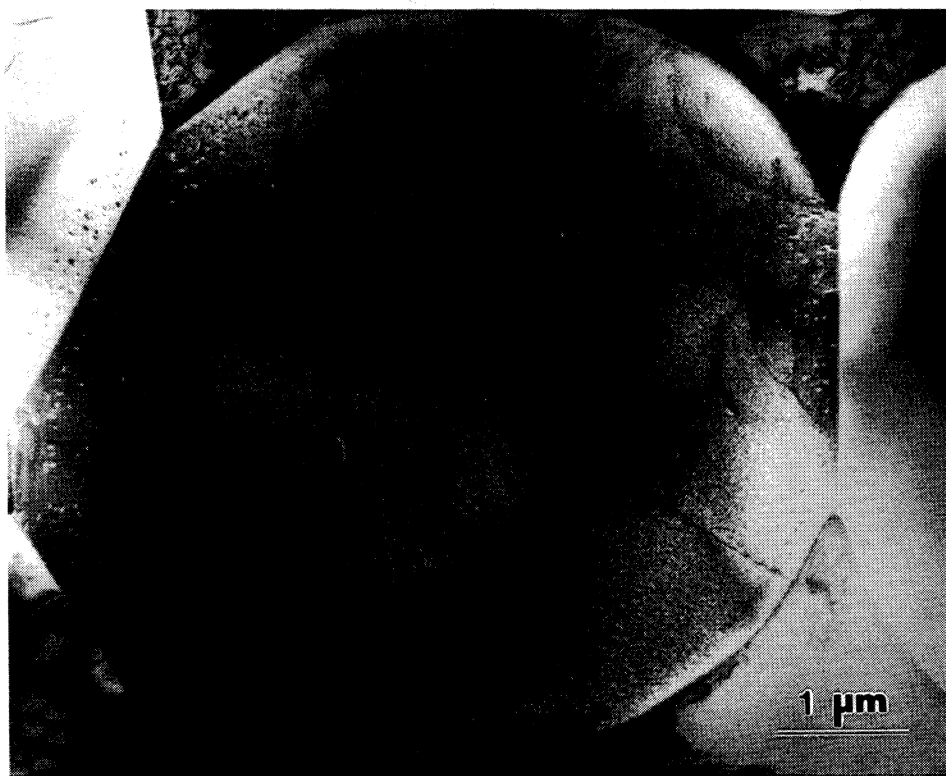
Fig. 13. Low dislocation density within a TiC grain (TEM).
