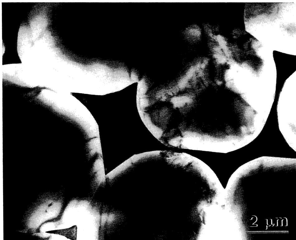
Fig. 12. Faceting of the TiC phase within the TiC-30Ni material (TEM).
