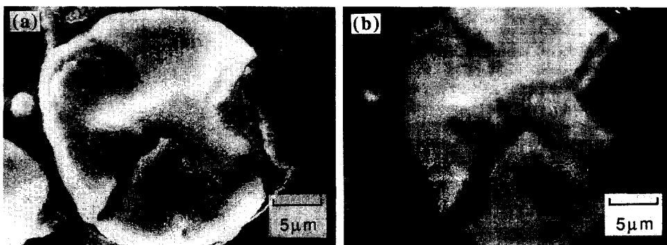
Fig. 5. (a) Scanning electron micrograph of polished or fractured TiC particle cross section, and (b) corresponding backscattering electron image.
