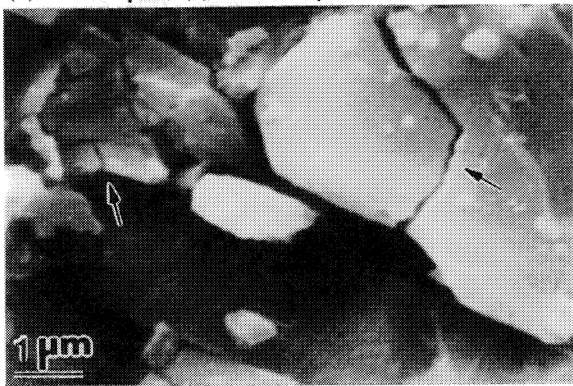
FIGURE 6. Detail of particle fracture (arrows) in regions adjacent to shear band.
