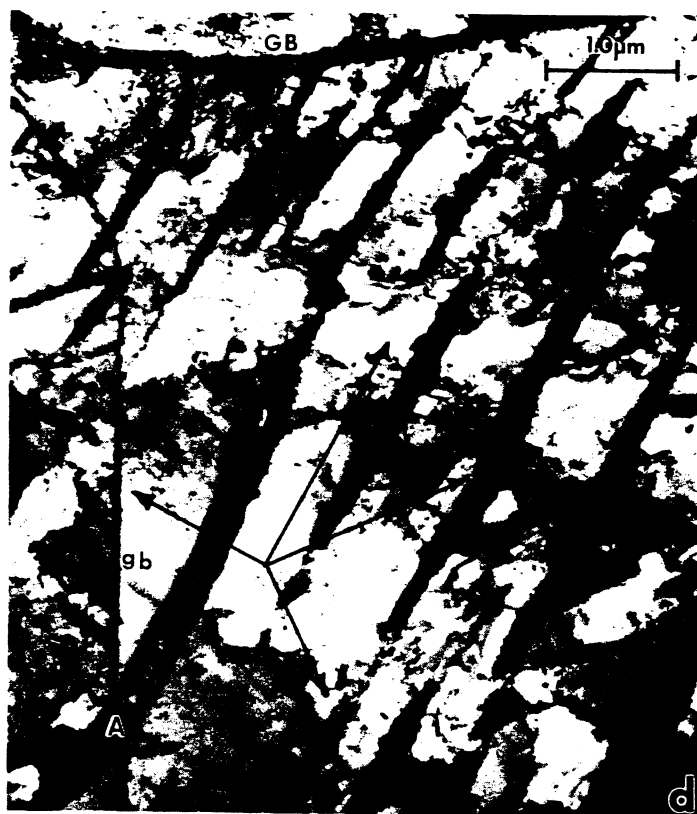
Fig. 1: Comparative views of starting Ta liner materials and plane-wave, shock-loaded Ta plate. (a) Light micrograph of typical Ta shaped charge (annealed) liner showing equiaxed grain structure. (b) Typical TEM view showing grain boundary triple point in liner material in (a). (c) Light micrograph of plane-wave, shock-loaded (45 GPa) Ta plate. (d) TEM image of deformation twins in (c). The grain surface orientation in (d) is (100). The principal \langle 042 \rangle directions are shown by arrows. The twin boundaries lie along these trace directions coincident with \{112\} planes which make an angle of roughly 66^\circ with the grain surface. Note high-angle grain boundary at GB and low-angle boundary at gb which is "sheared" as it crosses the deformation twin at "A".
