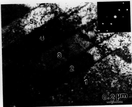
Figure 6 TEM at the region of \sim 1.5 \text{ mm} from center ( \epsilon_{\text{eff}} \approx 1.8 ; 400 K); SAD from cell 4.
