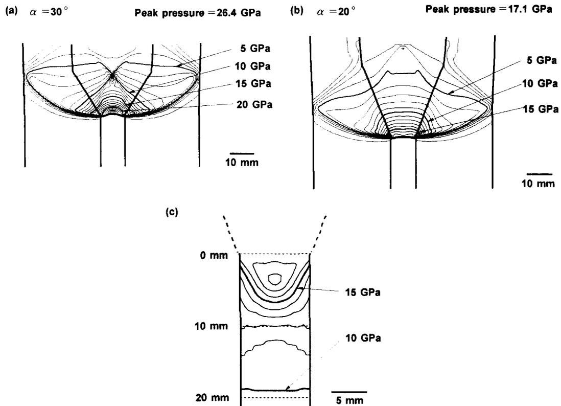
Fig. 3. Calculated water pressure distribution just above powders (converging angle =  $30^\circ$  (a) and =  $20^\circ$  (b)), and maximum pressure distribution in powder part (c).
