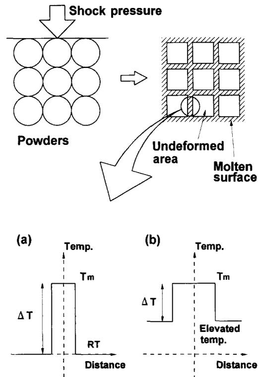
Fig. 5. Schematic illustration for formation of melting layer for room (a) and high-temperature (b) shock consolidation.
