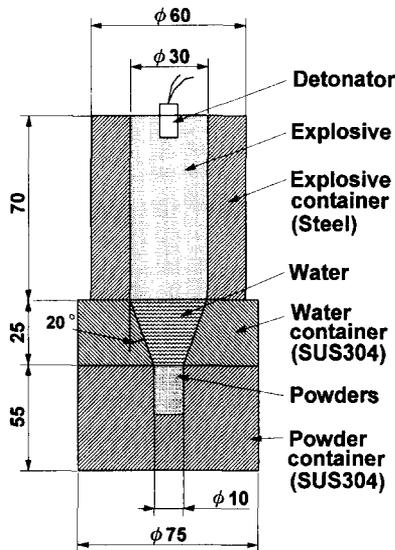
Fig. 2. Details of assembly.
