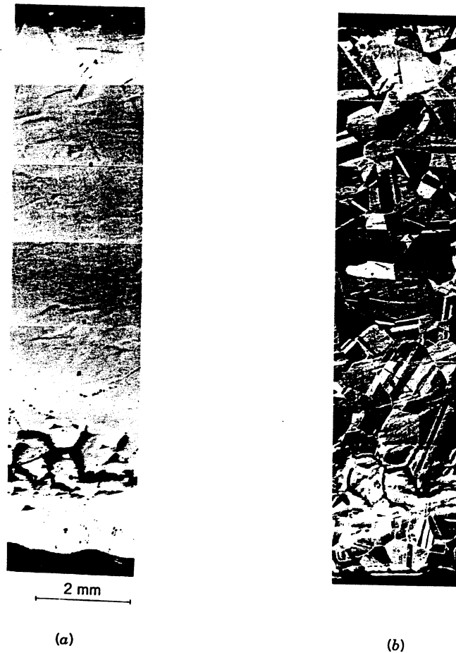
Figure 14.53 Cross section of copper specimen impacted by planar-parallel flyer plate, generating pressure of 3.5 GPa: (a) unetched specimen; (b) etched specimen.
