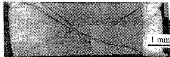
Fig. 4. Tantalum specimen tested in compression to a total strain of -0.6 at 77 K and 5500 s^{-1} .
