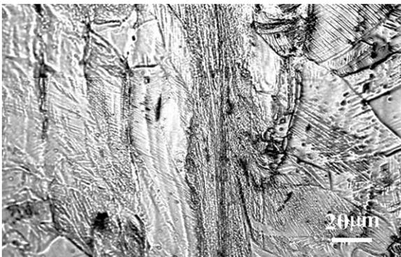
Fig. 2. Microstructure of shear band in stainless steel 304L produced in a hat-shaped specimen.
