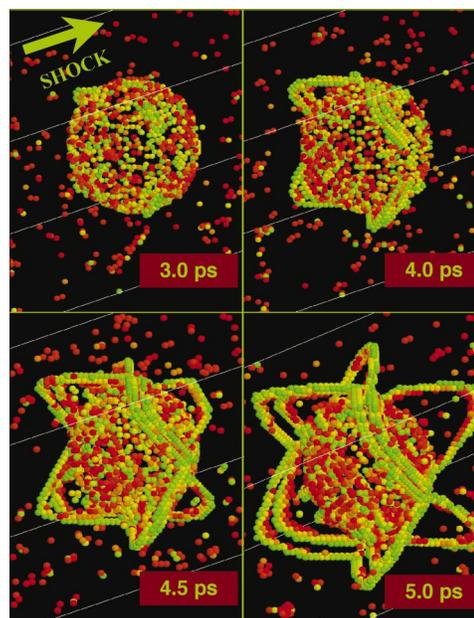
FIG. 1. (Color) Snapshots from an MD simulation, showing evolution of void collapse for a shock of 8 GPa and a void radius  $R=1.5$  nm ( $\sim 1200$  vacancies). Only defective atoms are shown. Numbers in boxes indicate time in ps after shock was applied; emission of loops starts at 3 ps.
