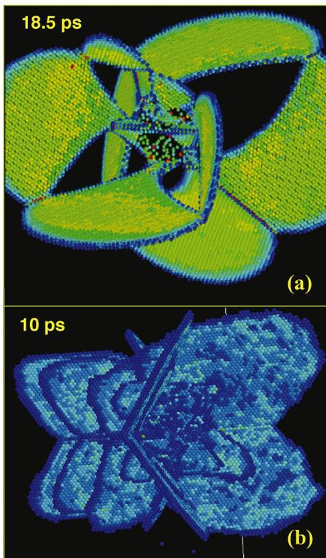
FIG. 2. (Color) Snapshots from an MD simulation for a void with  $R = 2$  nm ( $\sim 2850$  vacancies). (a) 8-GPa shock. Shear loops grow with a velocity  $v/c_0 \sim 0.15$ , where  $c_0$  is the sound speed at normal conditions. Snapshot from a similar MD simulation for (b) a 21-GPa shock. Loops grow at nearly the sound speed  $c_0$ . In both (a) and (b) only defective atoms are shown.
