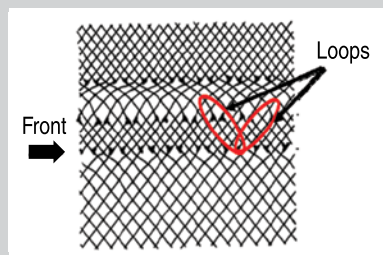
Figure 5. Shock compression of Ni along [001]; (a) Molecular dynamics simulation of stacking faults, viewed along longitudinal z direction. (b) Plastic and elastic zone formation; notice the formation of partial dislocation loops. (Figure adapted from Jarmakani et al. 10 ) (c) A dislocation interface in the homogeneous generation mode. (Figure adapted from Meyers. 11 )
