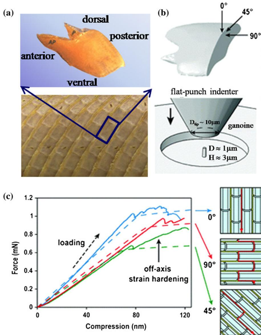
Fig. 7. Structural details and mechanical performance of Senegal bichir fish scale (adapted from Ref. 16): (a) scales; (b) nanopunch test setup on ganoine portion of scale using specimen with a diameter of  $1\ \mu\text{m}$  and a length of  $3\ \mu\text{m}$ ; and (c) force-displacement curves of ganoine along different orientations; red lines indicate crack paths between mineral crystals.
