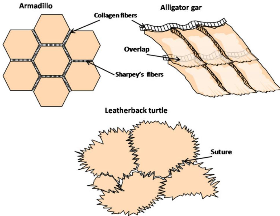
Fig. 3. Three different strategies to provide flexibility: collagen fibers connecting juxtaposed hexagonal osteoderms in armadillo, overlap between bony scales in alligator gar, and suture between osteoderms in leatherback turtle plastron.
