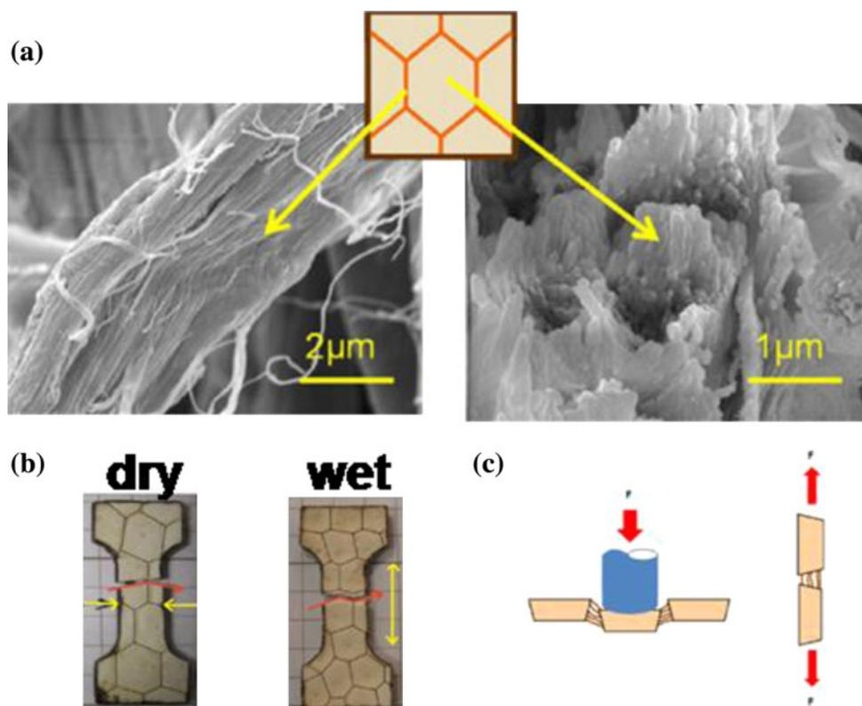
Fig. 8. Structural details of armadillo (adapted from Ref. 12): (a) nonmineralized collagen fibers between osteoderms (Sharpey's fibers) and mineral configuration in a deproteinized osteoderm; (b) fracture paths in dry (left) and wet (right) specimens; and (c) shear and tensile loading of osteoderms creating tensile loading of Sharpey's fibers.
