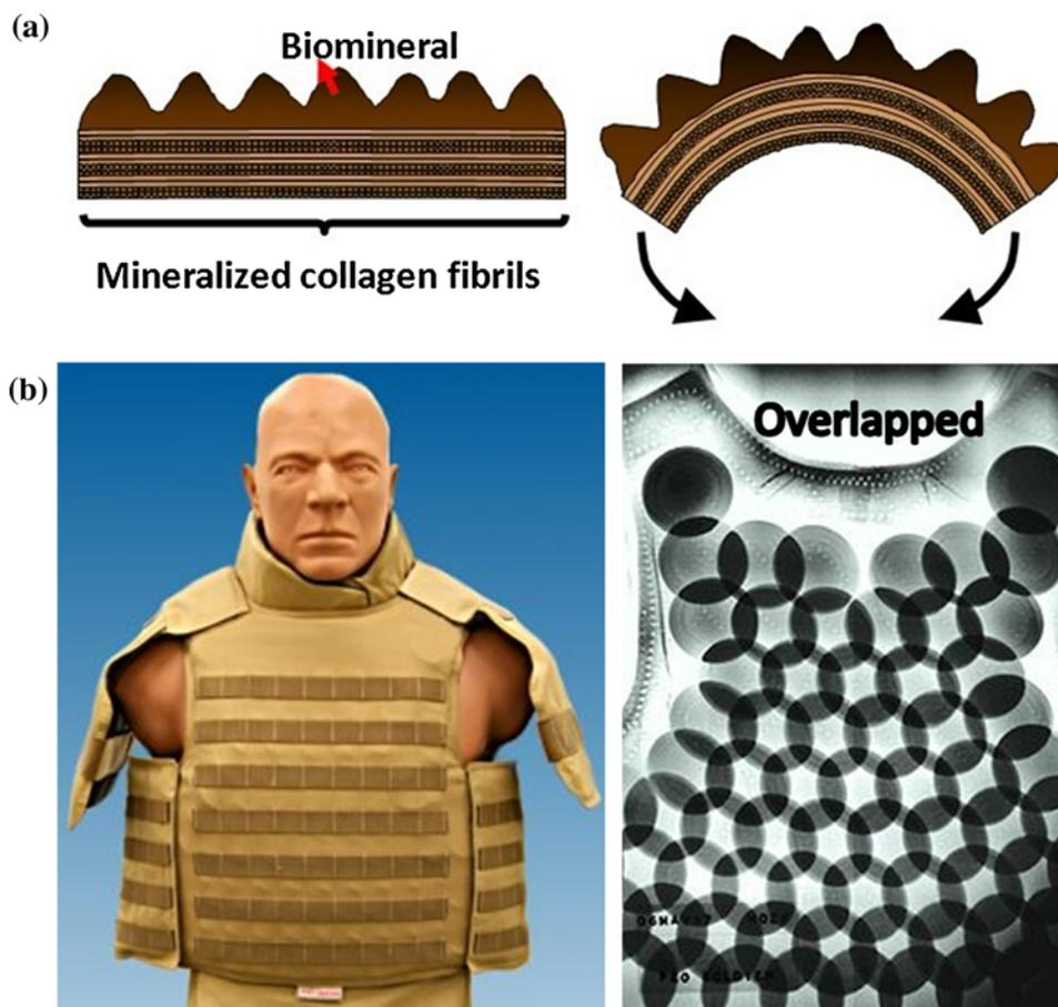
Fig. 10. Bioinspired flexible dermal armor: (a) conceptual view of flexible ceramic using arapaima scales as bioinspiration;<sup>17</sup> corrugations in ceramic decrease deleterious effects of tensile stresses; and (b) “Dragon Skin” armor.<sup>20</sup>
