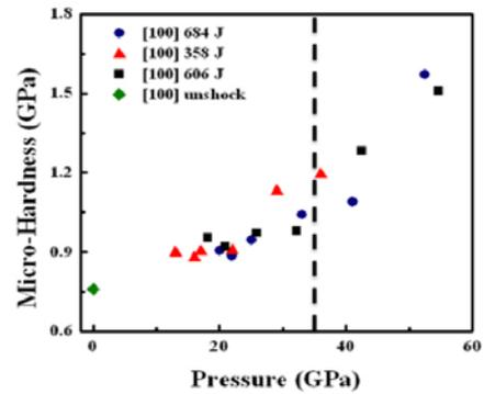
**Figure 6.** Hardness vs. pressure for all five experiments; notice increase beyond 35 GPa from twinning.
