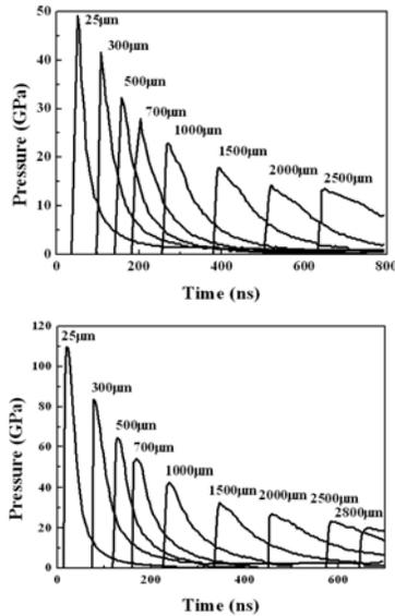
**Figure 3.** LASNEX simulations of the decay of the laser-generated pressure pulse as it travels through [100] tantalum specimen for (a) total laser energy of 358 J; (b) and total laser energy of 684 J.
