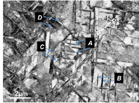
**Figure 5.** Twins imaged by SEM-BSE (20 kV) in [100] Ta at laser energy of 606 J; (~ 590 μm from laser shock surface).
