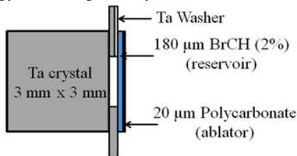
**Figure 1.** Monocrystalline Ta specimen and laser energy deposition assembly for quasi-isentropic compression.
