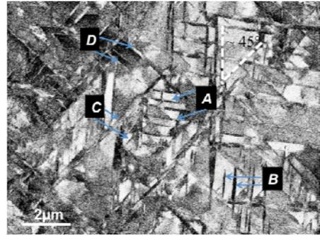
**Figure 5.** Twins imaged by SEM-BSE (20 kV) in [100] Ta at laser energy of 606 J; (~ 590 µm from laser shock surface).
