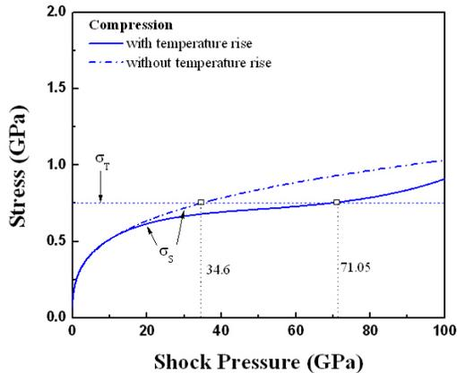
**Figure 8.** Slip and twinning stress is a function of shock pressure. The slip-twinning transition is in range 35-70 GPa.
