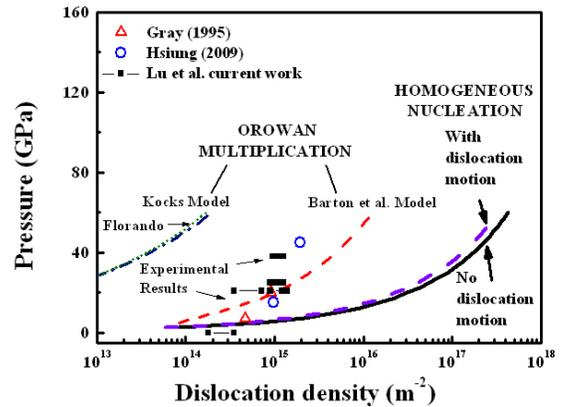
**Figure 7.** Dislocation density calculated from TEM images vs. Pressure and comparison with Orowan equation.
