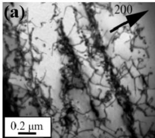
**Figure 4.** TEM micrograph at a distance from the laser deposition surface of 1.3 mm for [100] Ta single crystal, driven with laser energy of 606 J.
