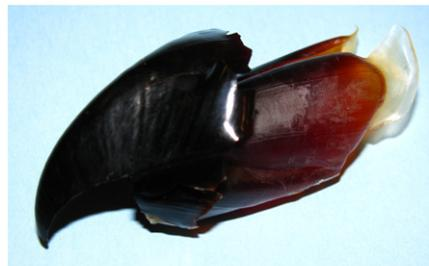
**Fig. 133.** (a) Squid beak (black) embedded in body (lighter); nanoindentation hardness of two regions marked; (b) beak extracted from animal showing gradient in tanning.
