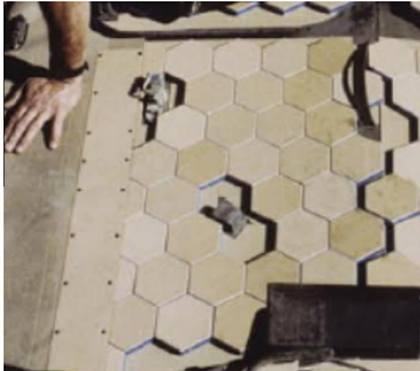
**Fig. 180.** LAST army tiles on an army tactical vehicle. These LAST<sup>®</sup> tiles have a ceramic interior and are coated with a polymer (picture taken from (<http://www.foster-miller.com/literature/documents/LASTGround.pdf#LASTGround>)).
