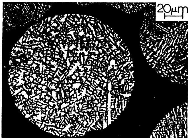
Figure 2. Cross-section of particle showing dendritic structure.
