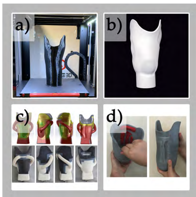
Fig. 8. Examples of prosthetic sockets manufactured with different AM technologies: a) FDM b) SLS © 2007 Rogers et al. [33]. Reprinted by Permission of SAGE Publications, Ltd. c) Inkjet © 2013 Wolters Kluwer Health, Inc. Reprinted with permission from Sengeh and Herr [46]. d) Multi-material printing © 2015 Comotti et al [47]. Reprinted with permission from Association for Computing Machinery.
