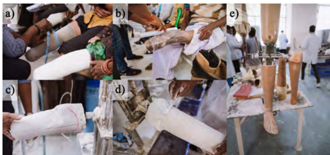
30 31 32 33 34 35 36 37 38 39 40 41 Fig. 3. Traditional process for manufacturing prosthetic limbs. a) Measuring key patient features. b) & c) Creating a plaster cast of an amputee's limb. d) Shaping the plaster limb cast. e) Manufacturing and adjusting final prosthetic socket
