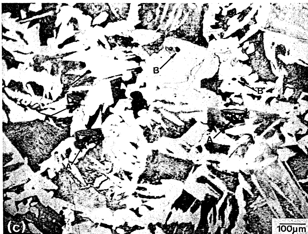
FIG. 33. (a) Crack propagating through pearlite colony; notice that crack stops in ferrite grain (SEM). (b) Cracks in steel propagating in brittle mode and joining second-phase particles (SEM). (c) Three MnS particles (indicated by arrows) in whose surroundings damage can be seen. (Spec. A.)
