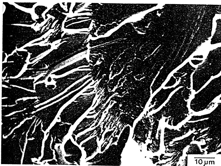
FIG. 39. Brittle fracture of steel in pre-shocked condition after impact in Charpy impact machine (SEM).
