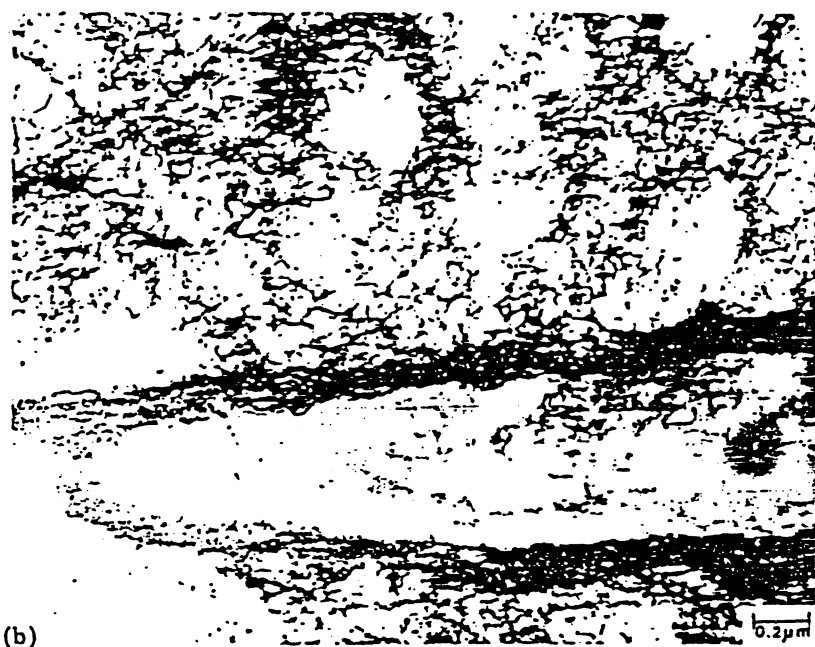
Fig. 13. Two transmission electron micrographs showing the breakdown of shock-wave-induced substructure occurring at the neck region of a tensile specimen (the effect of work softening).
