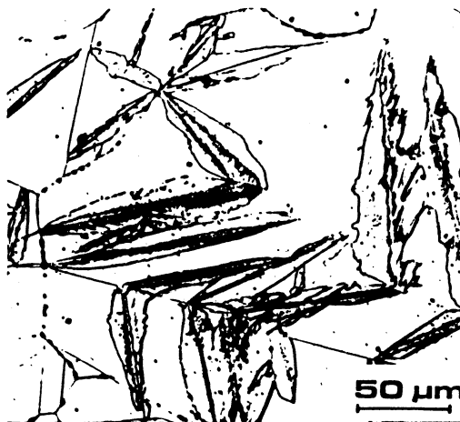
Figure 1. Optical micrograph of thermally induced martensite.
