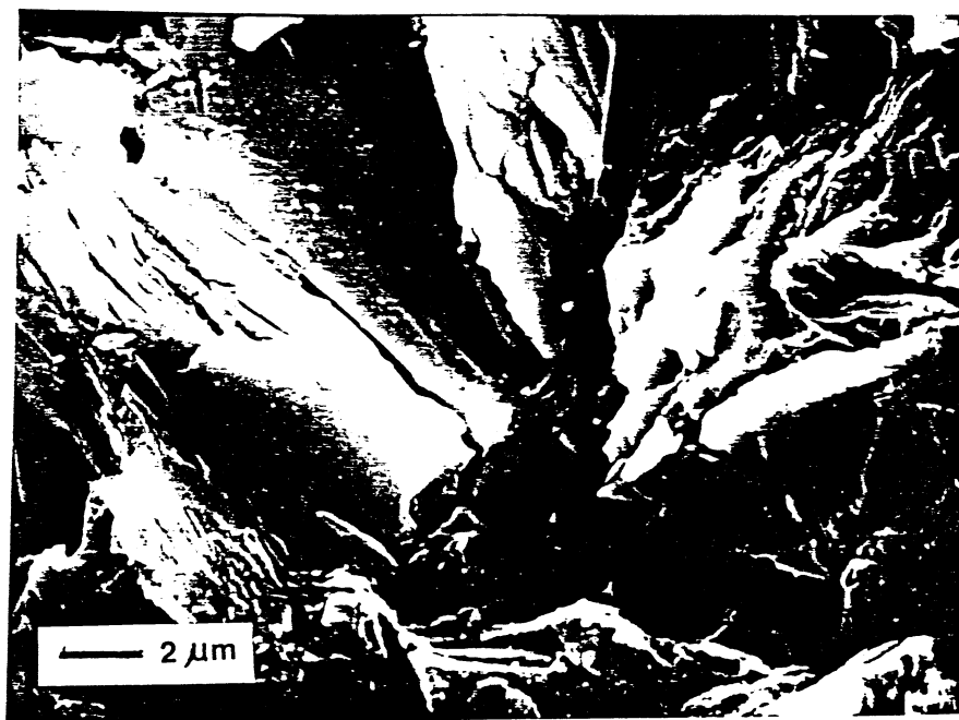
Figure 7. Intragranular and boundary cracks shown in sericite of Figure 6.
