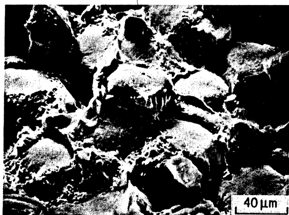
Figure 6 Appearance of tensile fracture region with tearing of interparticle melt regions.
