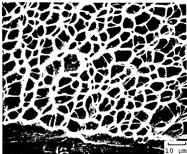
Fig. 11—Characteristic dimples observed in spall region of Ti6Al4V.
