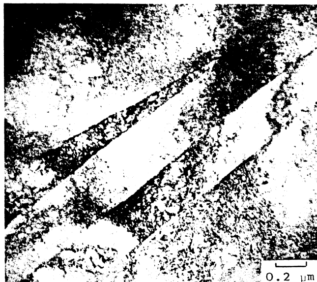
Fig. 15—Substructure produced by impact in titanium.
