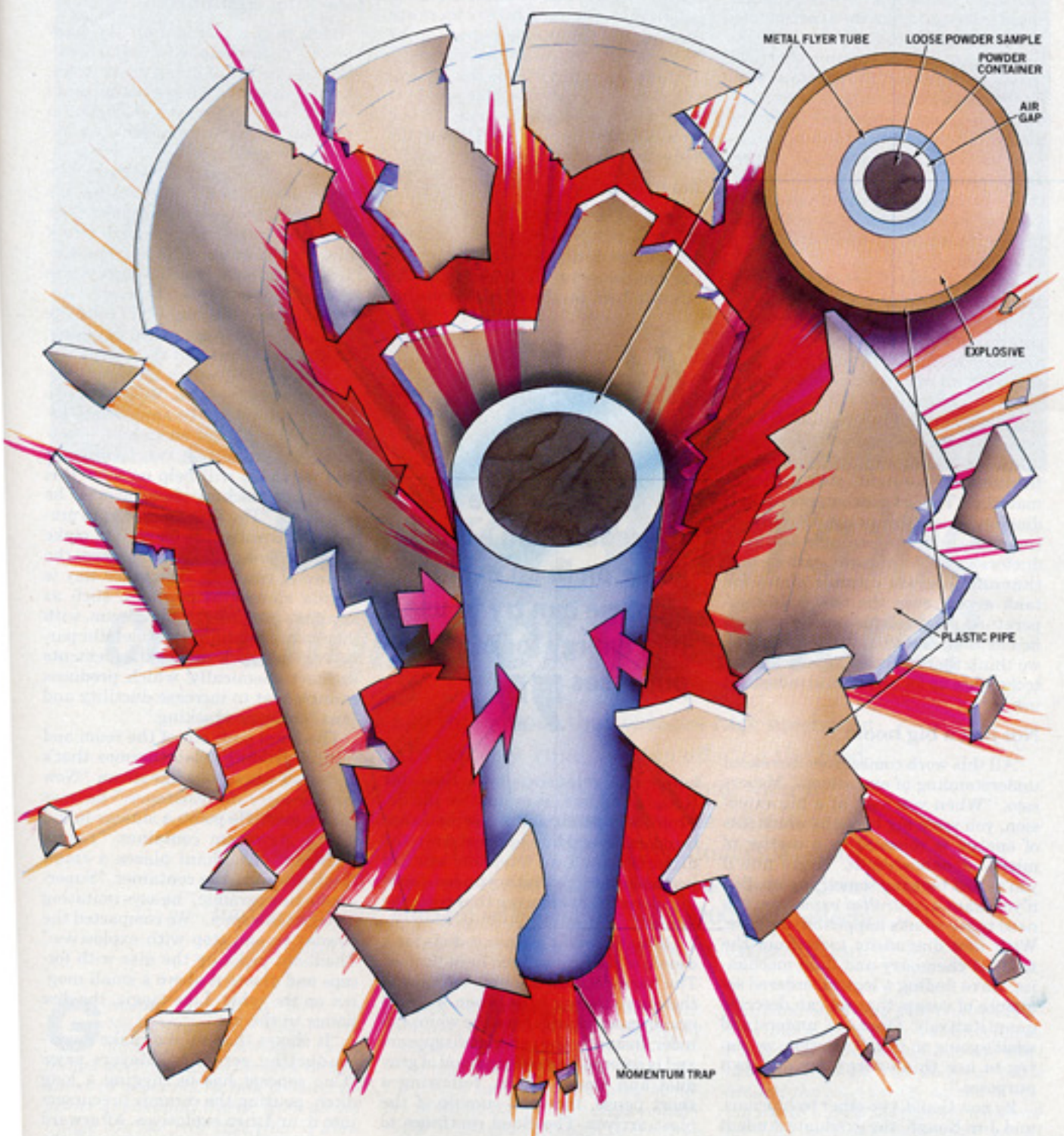
The cylindrical shock-compression apparatus shown above surrounds the powder sample with explosive pellets. Upon detonation, the explosives cause the sample material to implode, compacting the powder granules into a solid.
