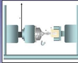
Fig. 3: Schematic of removal torque device. a. Vertical axis of universal test machine. Its vertical activation results in counter clockwise rotation. b. Insertion-removal key attached in the left grip. c. mini-implant inside the bone and the block attached in the right grip. The system maintains just a horizontal axis where the tests were realized.
