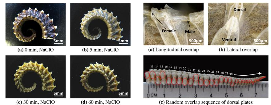
Fig 2. Time course of seahorse tail subjected to 12.5% NaClO in ambient conditions. Treatment used to determine the size, placement, overlap, and sequence of bony plates.
