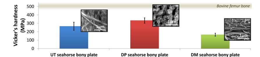
Fig 7. Micro-hardness and SEM insets of untreated (UT), deproteinated (DP), and demineralized (DM) seahorse bony plates compared to bovine femur bone. (All data from dorsal plates 13-19 at unspecified locations - see Fig 1).
