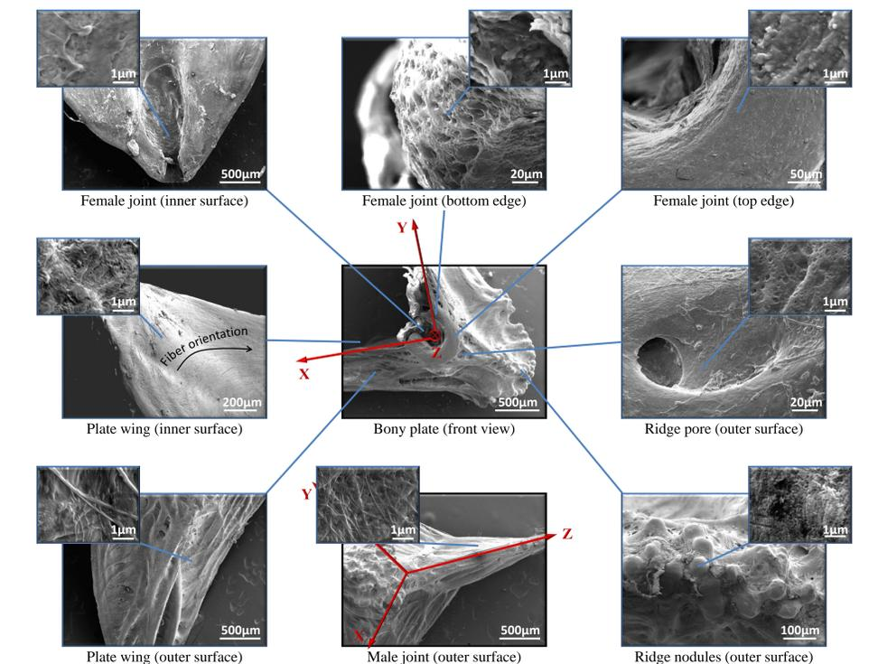
Fig 4. SEM micrographs of the untreated bony plates of a seahorse (*Hippocampus kuda*), illustrating the various surface features and roughness at several different locations, the 3-dimensional shape axes and the fiber orientation of the inner plate surface.
