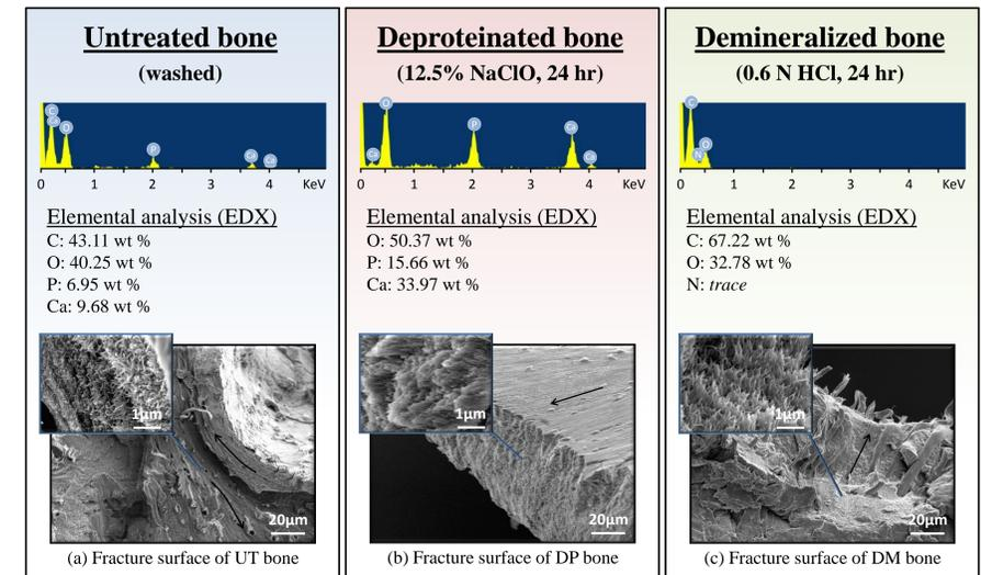
Fig 6. (Top) EDX elemental analysis and (Bottom) representative SEM micrographs showing fracture surfaces and fiber orientations of the plate wing of untreated (left), deproteinated (middle), and demineralized (right) bony plated armor.
