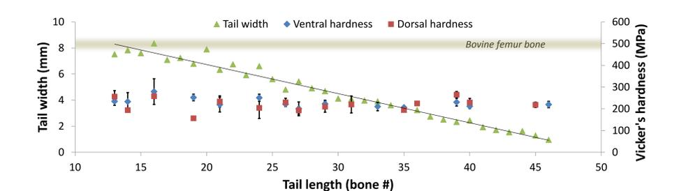
Fig 5. (Top image) Representative illustration of a bony plate and the measured micro-hardness (Vicker's hardness) at various locations (data from dorsal plates 13-19 - see Fig 1). (Plot) Tail width and micro-hardness of the bony plated armor (unspecified surface locations) versus seahorse tail length by bone # [5] (see Fig 1). Micro-hardness of bovine femur bone is shown for comparison.
