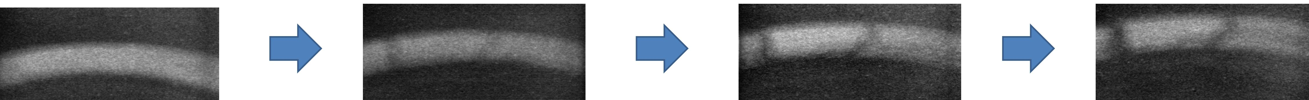
Swaged 100  $\mu\text{m}$  Aluminum powder ring w/ 18.8mm core
