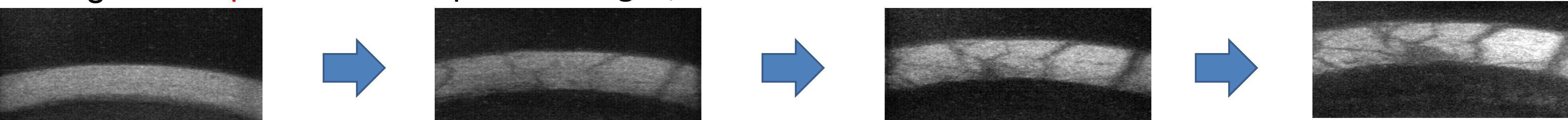
Swaged 100  $\mu\text{m}$  Aluminum powder ring w/ 12.7mm core
