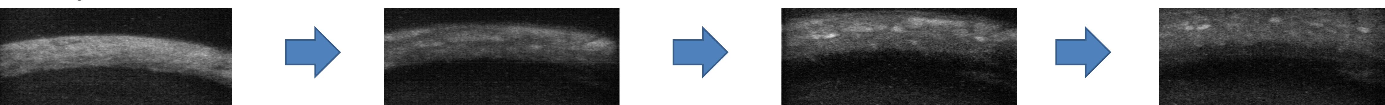
Swaged 40  $\mu\text{m}$  Aluminum powder ring w/ 18.8mm core
