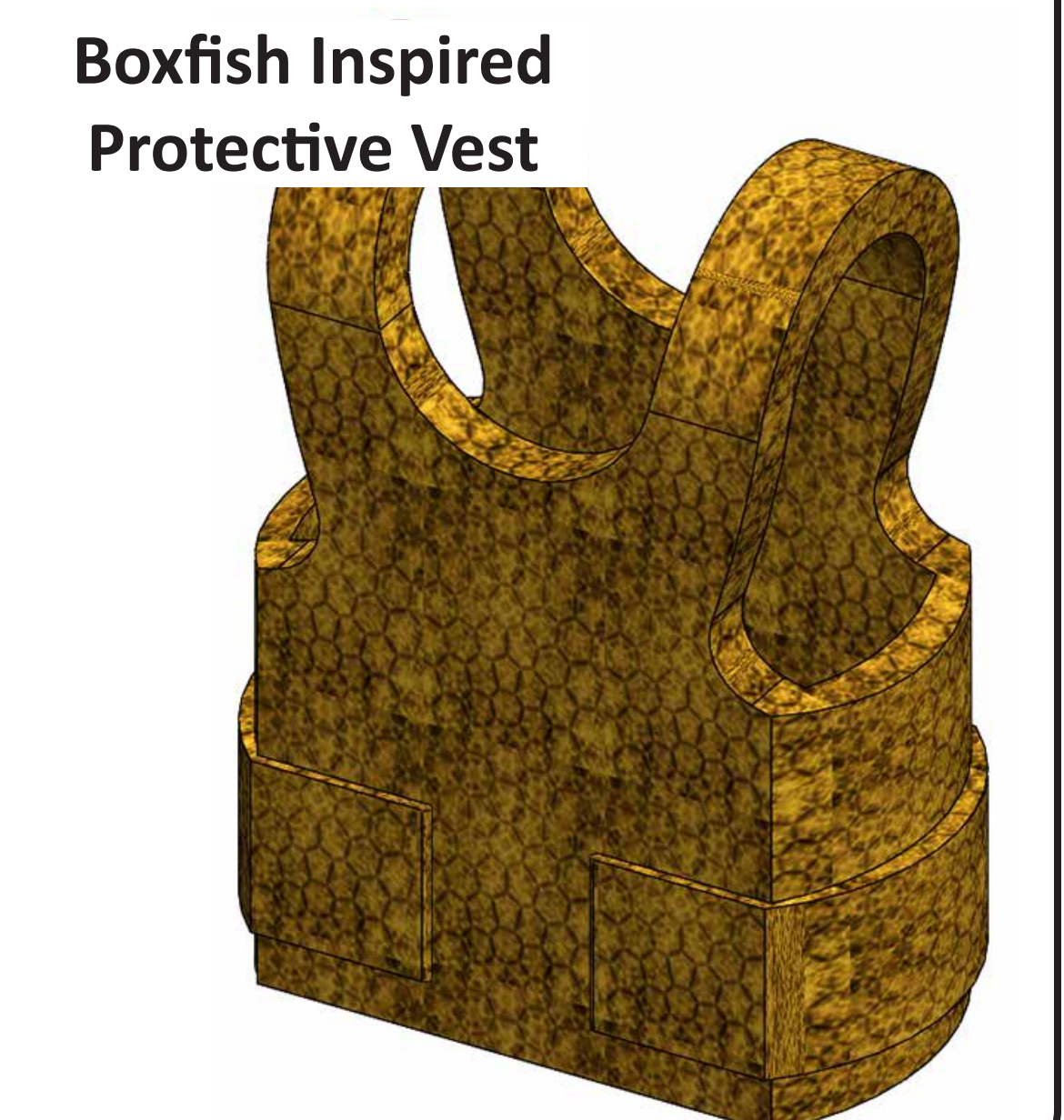
Bioinspired design based off of the boxfish scutes; (a) The boxfish scute, comprised of collagen and hydroxyapatite under assault from the piercing attack of fish teeth; (b) A bioinspired scute, comprised of stiff plate (e.g. steel) and a highly tough base (e.g. Kevlar) under assault from the piercing attack of a projectile.
