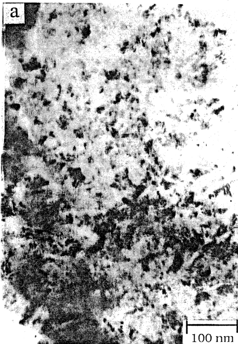
Figure 9a. TEM bright field micrograph of shear band material in the N-925 microstructure.
