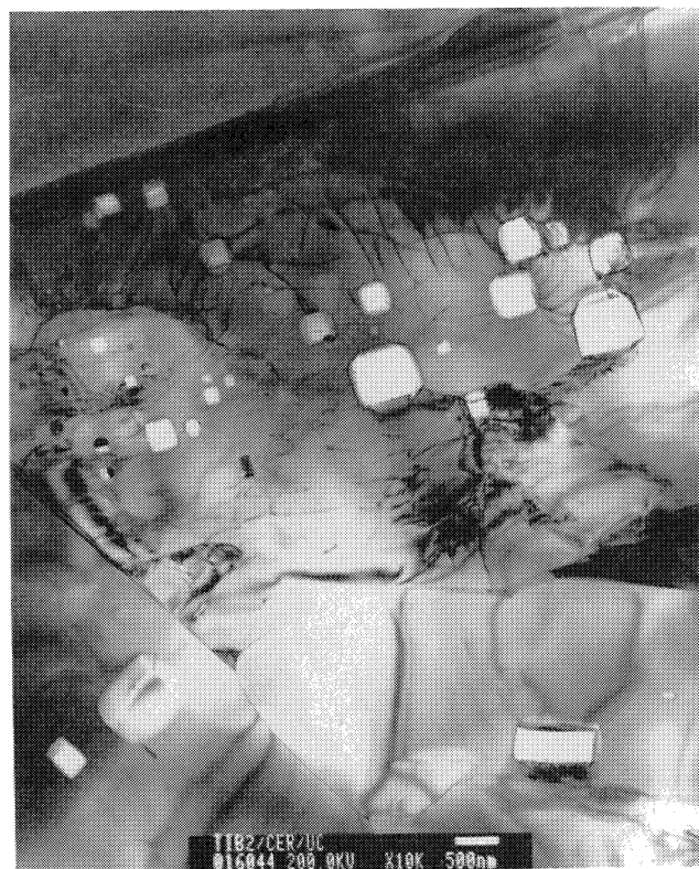
Fig. 10—Intragranular faceted voids in hot-pressed TiB 2 as viewed by TEM.
