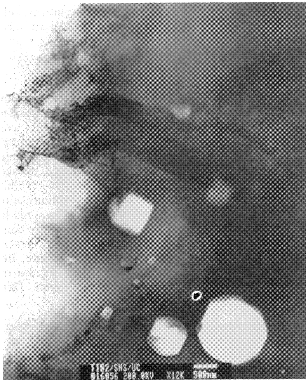
Fig. 7—Faceted intragranular voids in SHS/DC TiB 2 as viewed by TEM.
