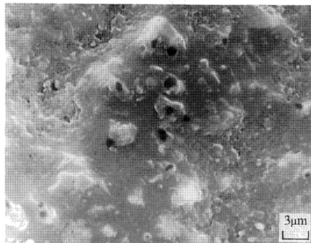
Figure 3 Scanning electron micrograph of polished surface of consolidated 4–8 \mu\text{m} diamond powders (1-1).
