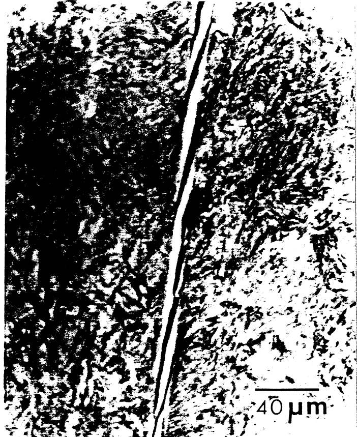
Figure 14 Crack and void formation along shear bands; (a) Ti; (b) Ti-Al-V alloy; (c) AISI1080, and (d) AISI 4340 alloy.
