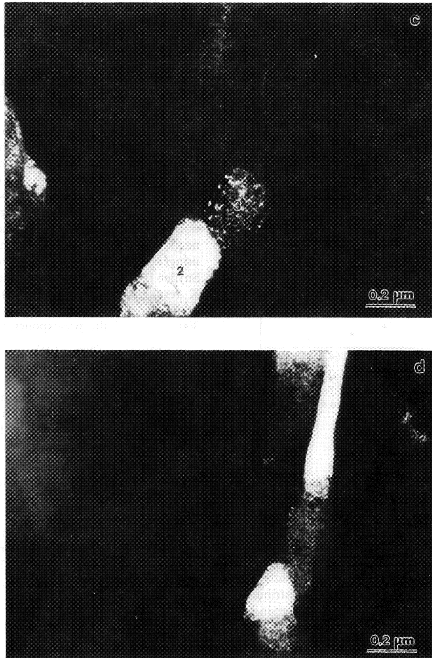
Fig. 16. (a) Bright-field and (b–d) dark-field images from a region < 0.5 mm from central axis showing recrystallized grains; notice grains 1-1, 2-2 and 3-3.
