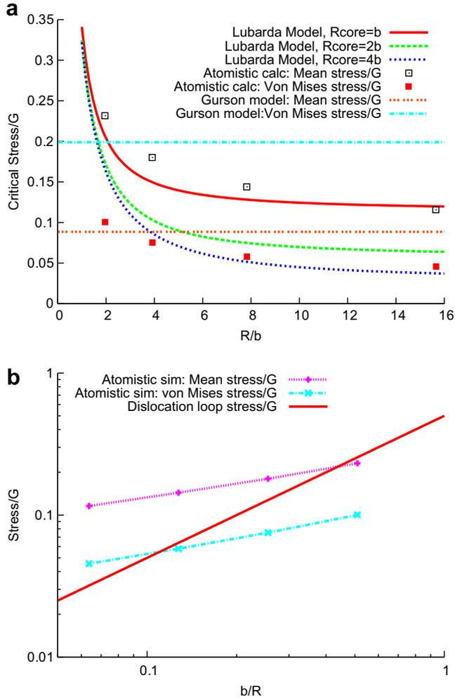
Fig. 4. Normalized critical stress against normalized void size: (a) with models and (b) on log–log scale.
