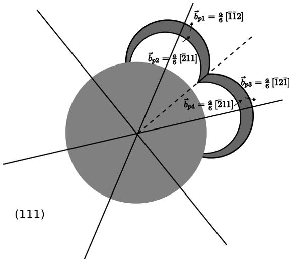
Fig. 6. In-plane partial dislocation interaction.
