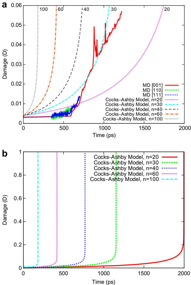
Fig. 15. Damage vs. time: (a) comparison of MD simulations and Cocks–Ashby equation and (b) predictions from Cocks–Ashby equation ( $n$  is exponent in power-law constitutive equation).
