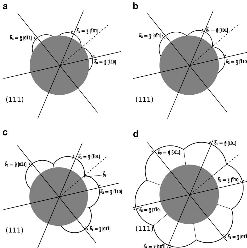
Fig. 5. In-plane dislocation interactions: (a) before interaction; (b) onset of interaction; (c) interactions and reaction and (d) uniform expansion of loops leaving dislocation segments behind.
