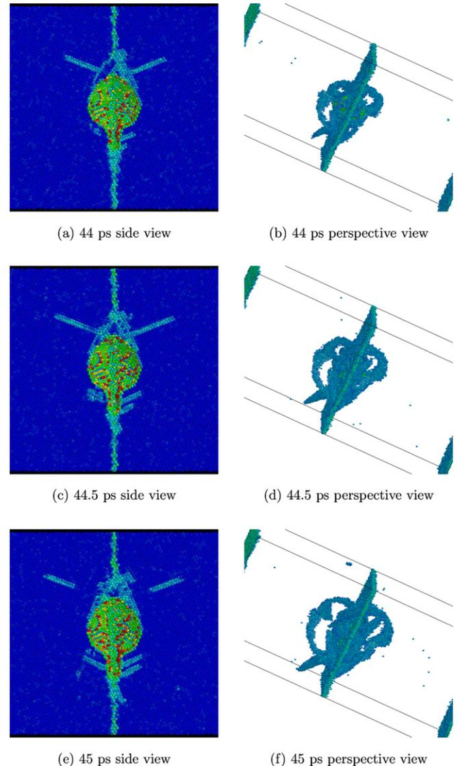
Fig. 12. Sequence of loop nucleation and growth in bicrystal simulation (times: 44–45 ps).
