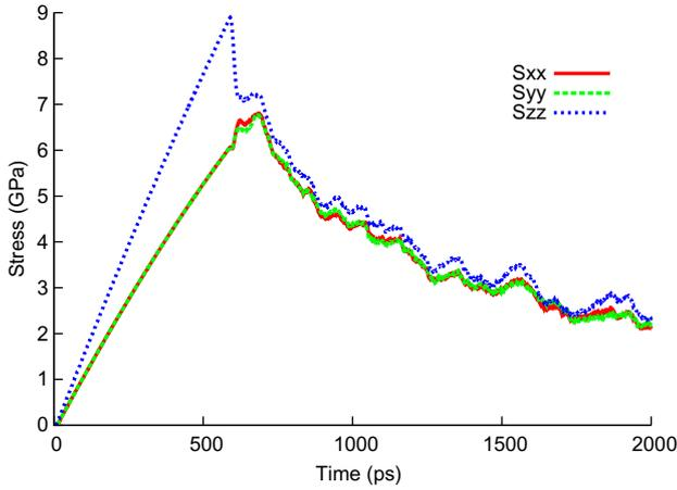
Fig. 13. Lateral stresses generated when loading is applied in direction ZZ.
