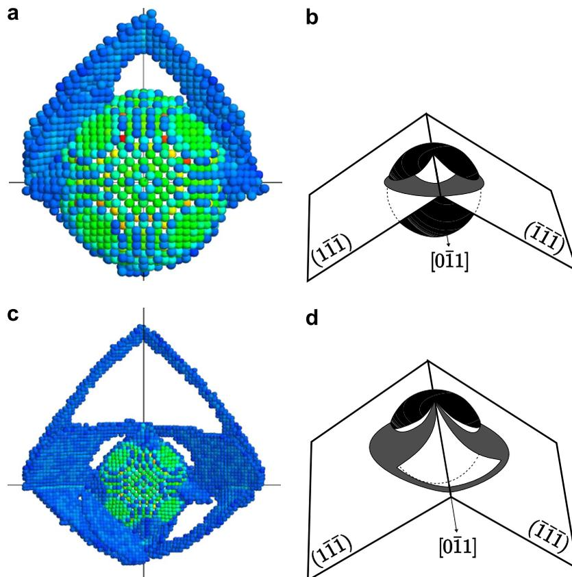
Fig. 8. Continued loop expansion: (a) rendered atoms from MD (591 ps); (b) corresponding sketched diagram; (c) rendered atoms from MD (595 ps) and (d) corresponding sketched diagram.
