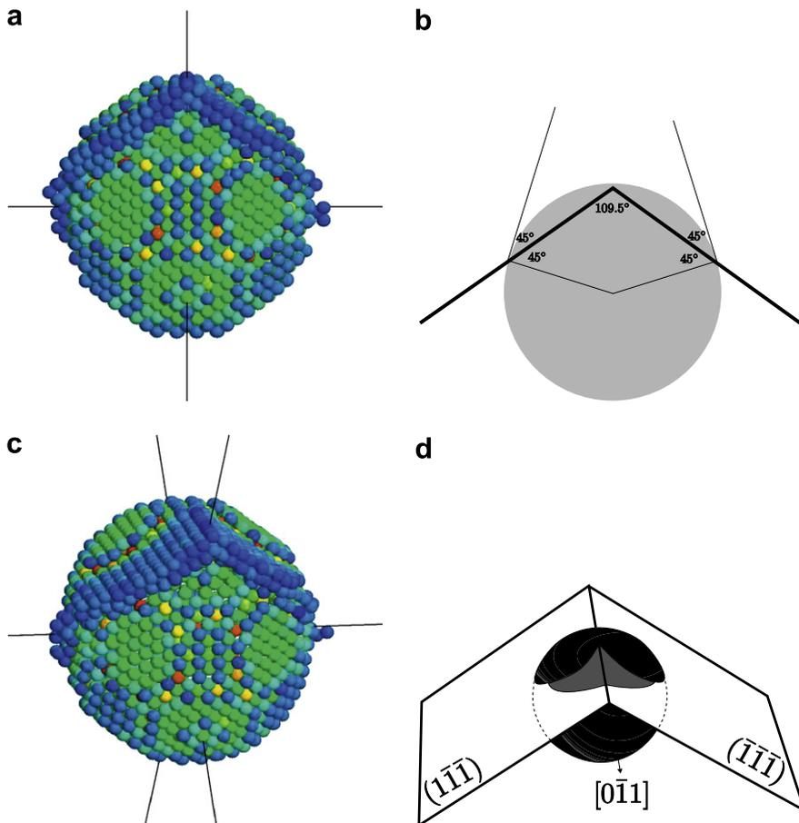
Fig. 7. Initiation of plastic flow at void surface (at 590 ps): (a) rendered atoms from MD; (b) diagram of (111) and (111) slip planes intersecting sphere surface at 45°; (c) rendered atoms from (a), rotated to show two loops and (d) diagram showing leading partial dislocations.
