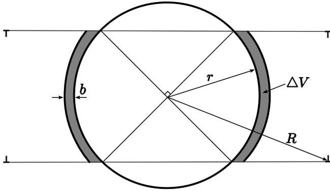
Fig. 16. Volume increment generated in void by the expansion of two shear loop rings.
