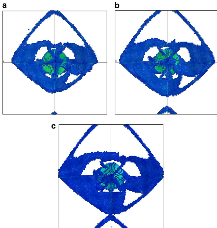
Fig. 9. Later growth and interaction of shear loops emanating from void: (a) 597 ps; (b) 598 ps and (c) 599 ps.
