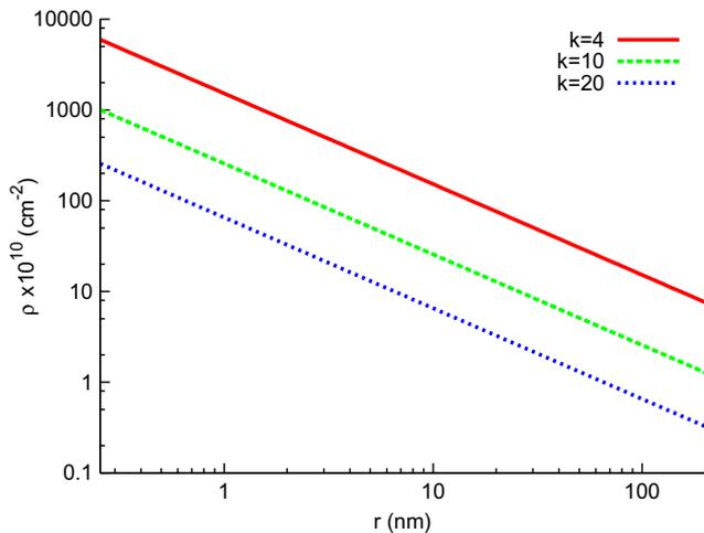
Fig. 17. Calculated density of geometrically necessary dislocations as a function of the ratio  $k = \frac{R}{r}$ .
