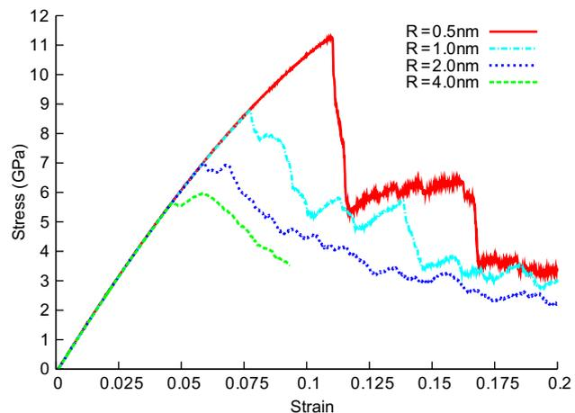
Fig. 3. Stress–strain relations for different void sizes, showing size-scale dependence of yield stress.
