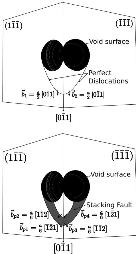
Fig. 14. Top view of loop interaction of biplanar dislocation loops on  $(1\bar{1}\bar{1})$  and  $(\bar{1}\bar{1}\bar{1})$ : (a) perfect dislocations and (b) partial dislocations.
