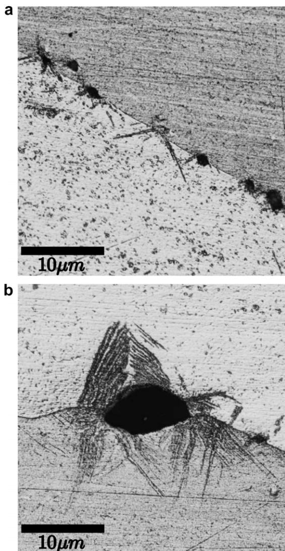
Fig. 2. Evidence of slip around growing grain-boundary voids: (a) Small voids and (b) large void.
