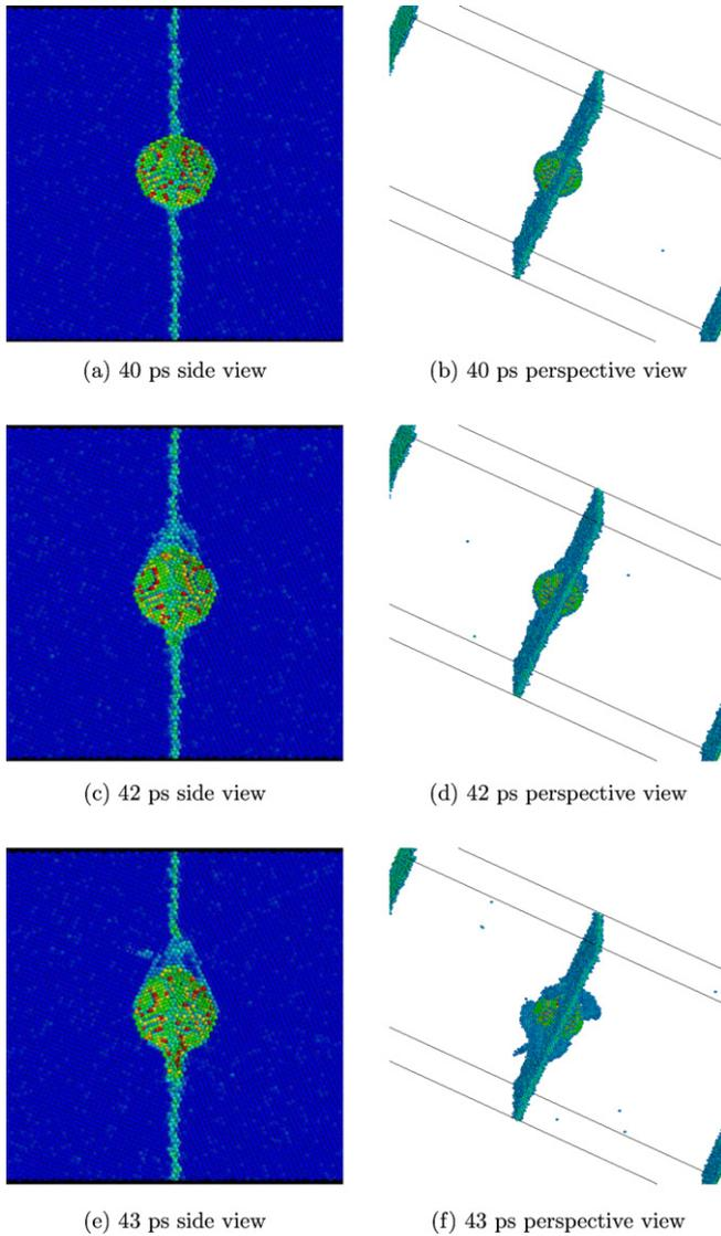
Fig. 11. Sequence of loop nucleation and growth in bicrystal simulation (times: 40–43 ps).
