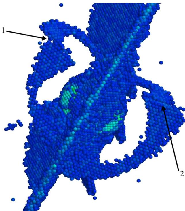
Fig. 10. Shear loops and their interaction in bicrystal simulation with initial void at grain-boundary (uniaxial strain).
