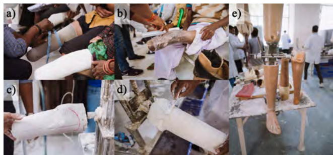
30 31 32 33 34 35 36 37 38 39 40 41 Fig. 3. Traditional process for manufacturing prosthetic limbs. a) 42 Measuring key patient features. b) & c) Creating a plaster cast of an 43 amputee's limb. d) Shaping the plaster limb cast. e) Manufacturing and 44 adjusting final prosthetic socket
