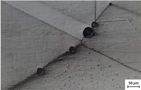
FIG. 3. Spalling voids in copper forming preferentially at grain boundaries.
