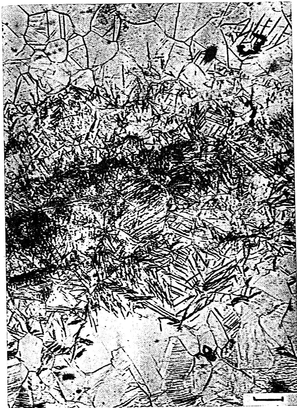
FIG. 2.25 Martensite generated by tensile hydrostatic stresses produced by a reflected pressure pulse in an iron-nickel alloy (from ref. 134). Bar = 100 \mu\text{m} .
