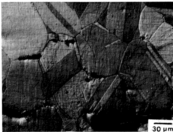
Fig. 8. Voids forming in copper due to tensile pulse produced by reflection of shock waves at a free surface; from (Christy, 1984).
