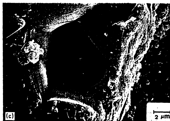
Figure 6 Cracks seen in impacted alumina at successively higher magnifications: (a) macrocracks; (b) mesocracks; (c) microcracks.
