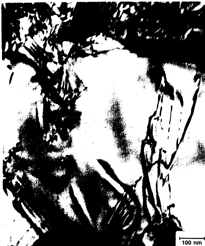
Figure 17 Dislocation in alumina impacted at 4.6 GPa in alumina capsule (compression + tension).
