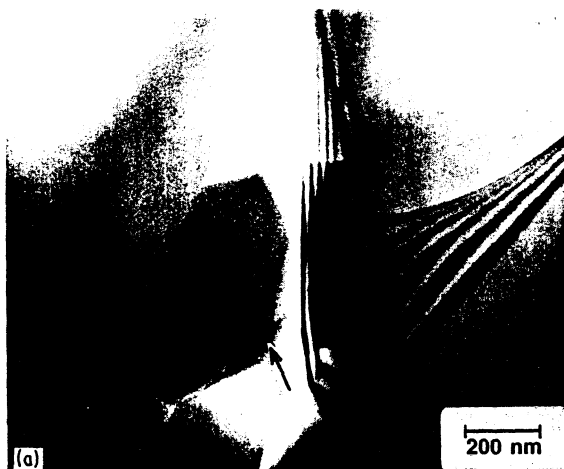
Figure 20 (a) Grain boundary and suspected cracks (arrowed) in alumina impacted at 4.6 GPa in aluminium capsule (compression + tension); (b) same area after tilting of specimen; notice disappearance of grain-boundary fringes.
