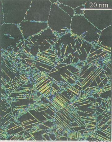
A COMPUTER simulation helped scientists at Lawrence Livermore Laboratory understand what effects a laser-induced shock wave traveling through nanocrystalline copper can have on hard metal.
